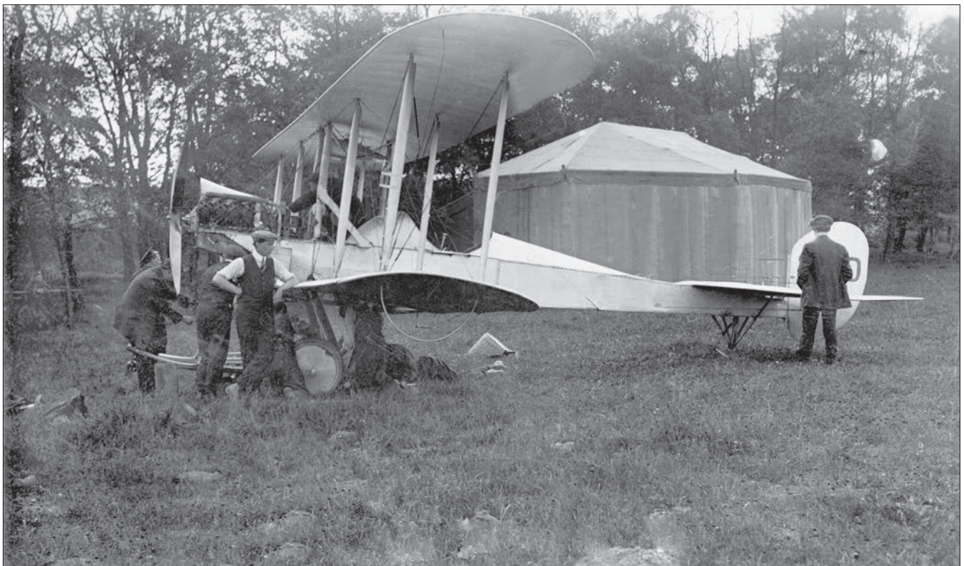
220, with a mechanic working on the generator that powered the wireless positioned behind the engine.
